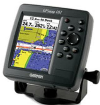
GPS is often quite accurate but both it and electronic charts are subject to errors. Sometimes the plotter can give a false sense of security as to your exact position so verify a GPS or plotter position with what you can actually see out the window and what your other instruments confirm. A 50-100m position error is a problem in a narrow channel but irrelevant at sea.
